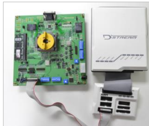
A9 Chip Testing Board
